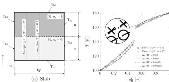
Figure 2. Left: Geometry and boundary conditions for a 2D slab problem; right: Exact and computed results.
