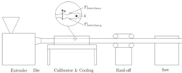
Figure 1. Schematic view of a thermoplastic profile extrusion line.
