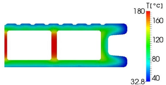
Figure 4. Temperature profile in the plastic after the calibration step.
