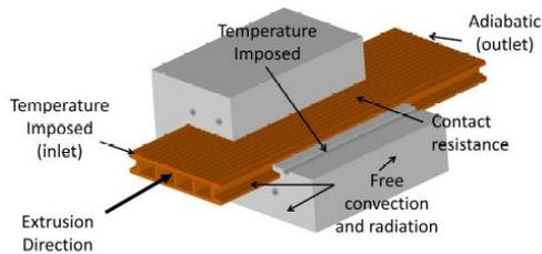
Figure 3. Complex plastic profile with thermal boundary conditions.
