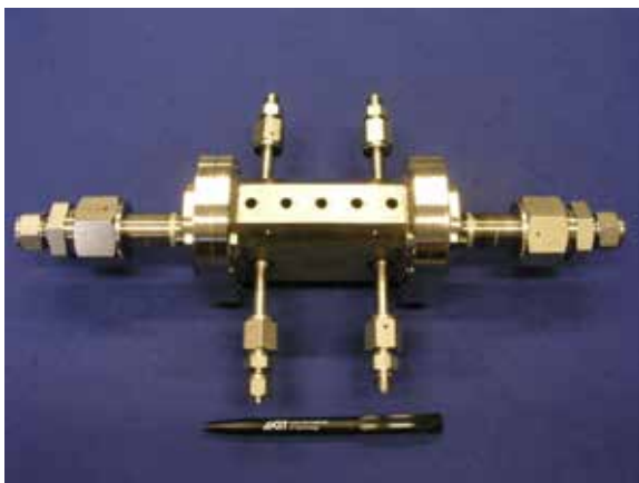
Figure 1. Microreactor prototype for mixed CO/CO 2 methanation.
