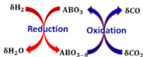
Figure 1. Two step RWGS-CL process for conversion of CO 2 to CO.
