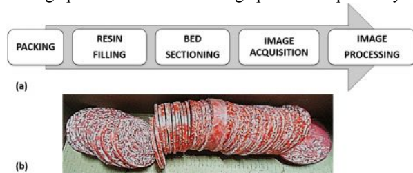
Figure 1. (a) Experimental methodology (b) Image of sliced column after bed sectioning
